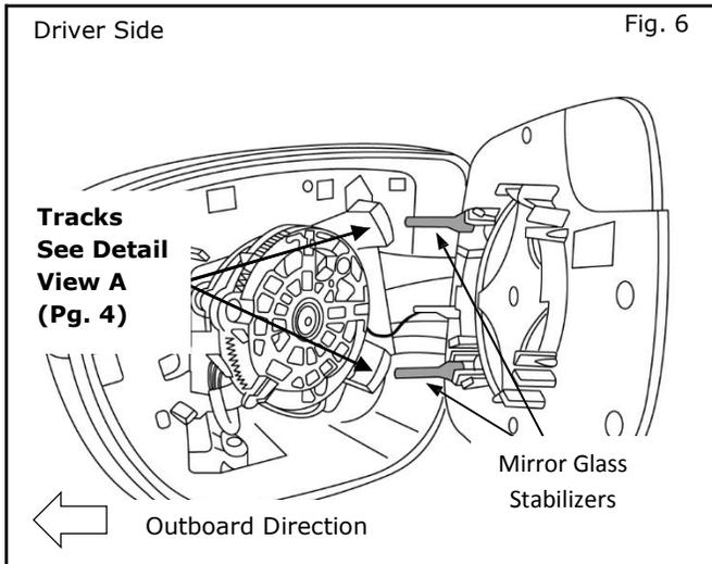
6) During glass installation, as BZM assembly is positioned within mirror housing, be sure two **mirror glass stabilizers** are lined up with **mirror stabilizer tracks** and make sure stabilizers are located on **OUTBOARD** edge of tracks.
