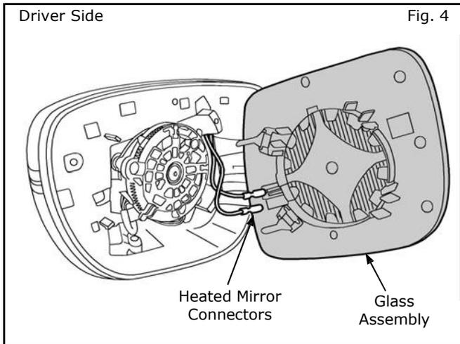
4) Carefully remove glass assembly from mirror housing.
