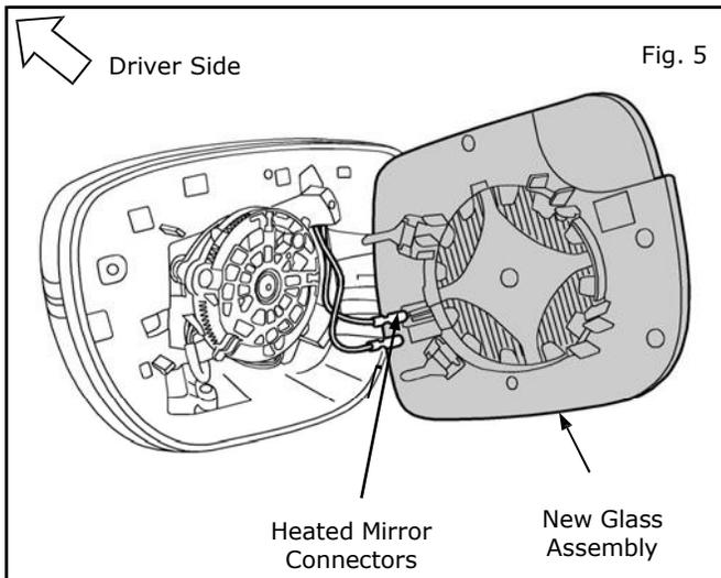
5) Begin installation of new Blind Spot Mirror Glass Assembly by reconnecting heater wires if necessary.
