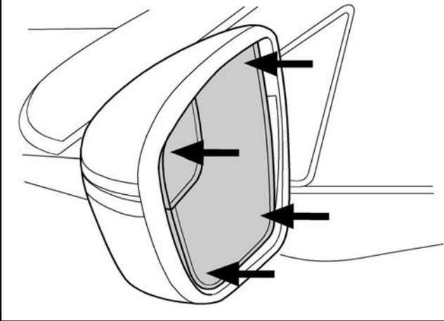
7) Using even pressure, press firmly on new glass assembly to seat it into mirror housing. Take care that initial force applied is **perpendicular** to Mirror Housing. You will hear and feel a definitive snap as mirror glass assembly engages with glass actuator.
